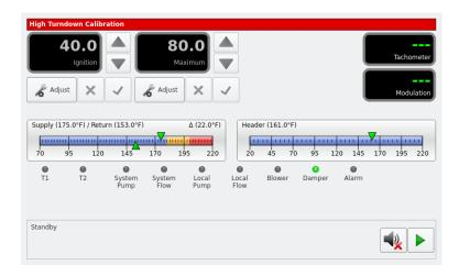
Pressing the Start Calibrate Button will allow the Min Air Shutter and Blower Clamp values to be set.
